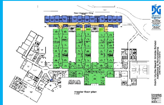
NMBM – Proposed Fire Sprinkler Add'n (in Green)
