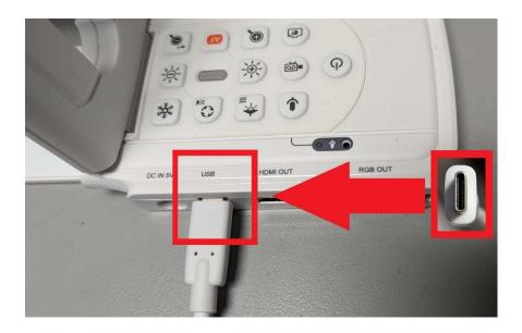
3. Plug the rectangle end into either USB port on the lower left of the Smartboard.
