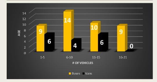
Note: Currently there are 9 spare buses and 2 spare vans. NWLSD replacement plan has been determined using a 15 year age for daily use vehicles in conjunction with mechanic analysis of fleet.
