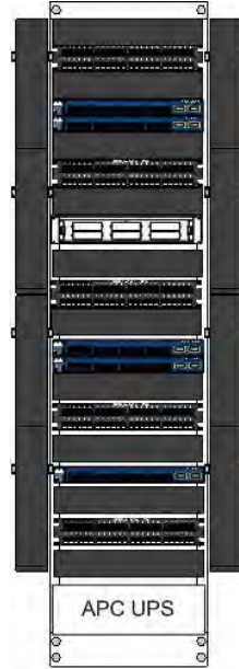
Typical ITR telecommunications rack layout
