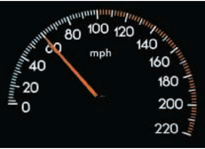
▲ FIGURE 2-6 A speedometer indicates a car’s instantaneous speed but gives no information about its direction . Thus, the speedometer is truly a “speed meter,” not a velocity meter.
