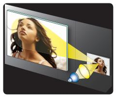
Most projection TVs are rear-projection systems; the image is displayed on the back of the screen and the projector is contained in the TV.
