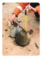
To test the consistency of concrete, inspectors perform a slump test by forming a cone of concrete and measuring how much it slumps due to gravity.
