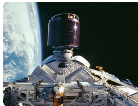
The SBS-4 communications satellite is deployed from the space shuttle payload bay.
