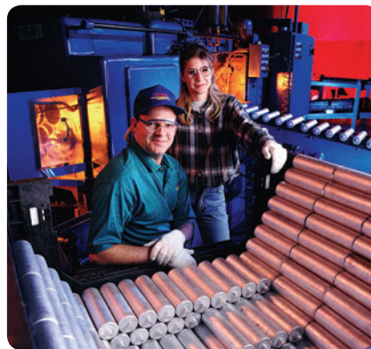
Two unionized workers inspecting air-bag canisters.
