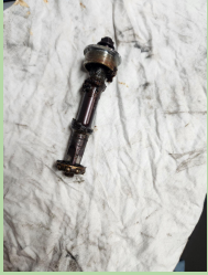
Bottom Bracket With Shredded Bearing
