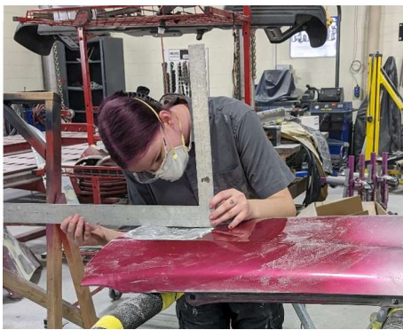
Collision Repair – Ashley Mullen (W) is checking steel for straightness while Jacob Allen (CM) and Evan Smith (PT) straightened a patch they welded in.
