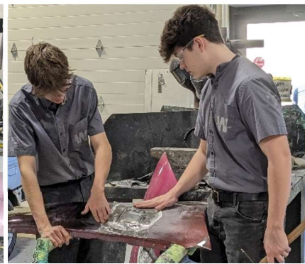
Collision Repair – Ashley Mullen (W) is checking steel for straightness while Jacob Allen (CM) and Evan Smith (PT) straightened a patch they welded in.
