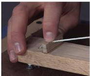
To tighten the strings, hold the wing nut and turn the eyebolt clockwise, wrapping the string around the eyebolt. Make sure the string is sitting in the grooves on the nut and the bridge. When the string is taut, firmly tighten the wing nut.
