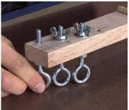
Repeat with the other two eyebolts. Lightly tighten all three eyebolts. The eyebolts should be placed in the holes corresponding to the red holes in the diagram at right. The string will pass through the holes marked in black, and attach to the bolts under the neck.
