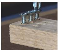
For each string, cut a piece of mason twine about 5 feet long. Tie the twine to the woodscrew. Thread the string through the empty hole next to the wood screw, over the groove on the bridge, along the neck, over the groove on the nut, and down through the corresponding hole next to the tuning peg. Then, double-knot the twine through the eyebolt.
