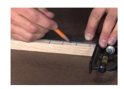
Next, make marks at the intersection of these lines, as in the diagrams. Then drill holes with a 1/4" bit.
