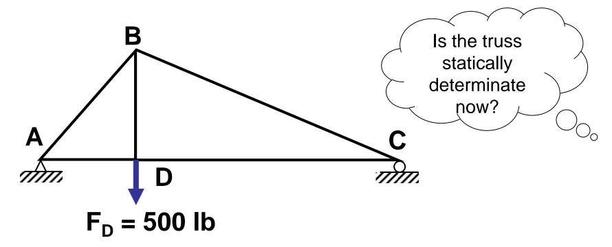
A truss is considered **statically** <u>determinate</u> when the static equilibrium equations can be used to find the reactions on that structure.
