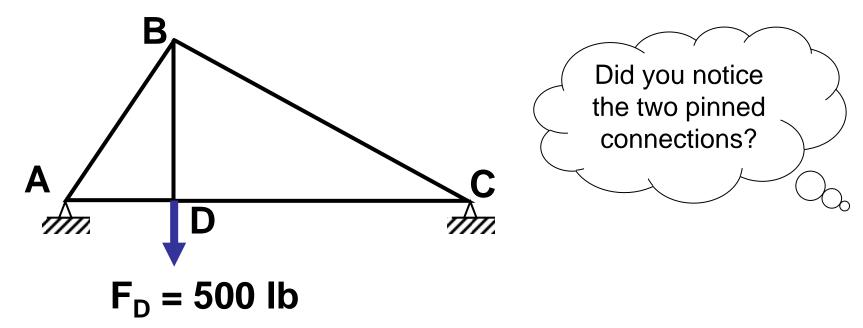
A truss is considered **statically** <u>indeterminate</u> when the static equilibrium equations are not sufficient to find the reactions on that structure. There are simply too many unknowns.
