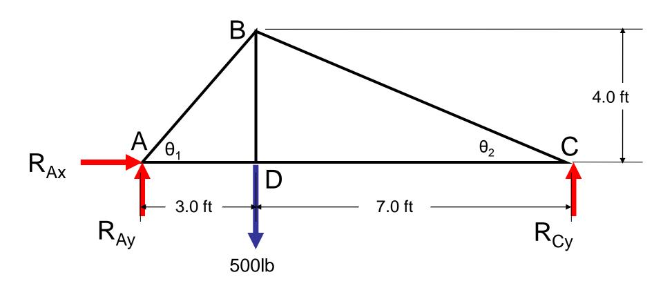
Using Truss Dimensions to Find Angles
