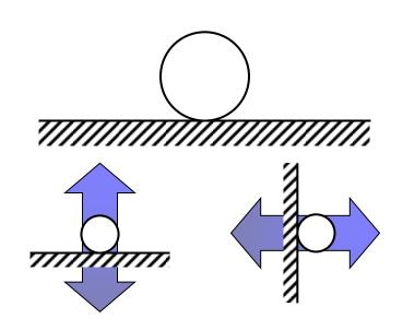
A **roller** support can support a structure in only one dimension.
