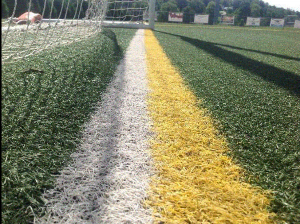
01. Fibers Laying Over and Coiling
