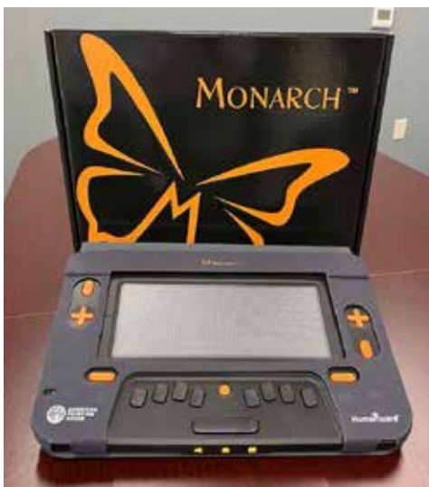
The Monarch device that Leslie, Susan, Nancy, and Erin each received along with technology training. Appropriately formatted tactile graphics can be displayed on the same unit which is capable of 10 lines of 32 cells of braille.
