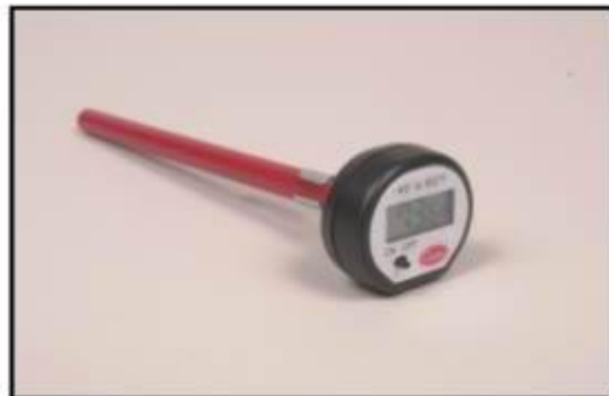
Digital Thermometer—for taking product temperature. Good for checking thin products such as hamburgers. Keep the digital display dry.
