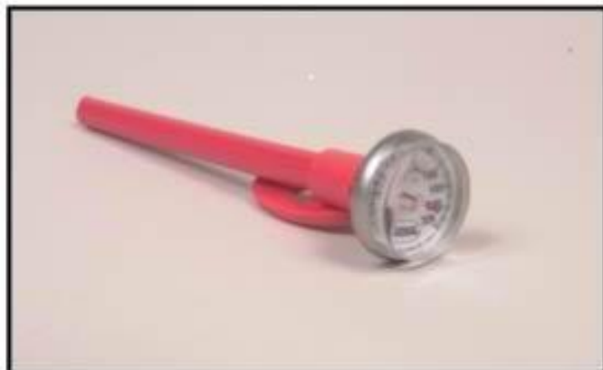
Bi-metallic Thermometer—for taking product temperature. Tip must be inserted at least 2" into food.
