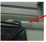
6. Tape the garbage bag at the top of the Promethean by placing the tape either on the back the Promethean system or to the frame as shown on the left. DO NOT PUT TAPE ON ANY PORTION OF THE FACE (WHITE PART) OF THE BOARD!
