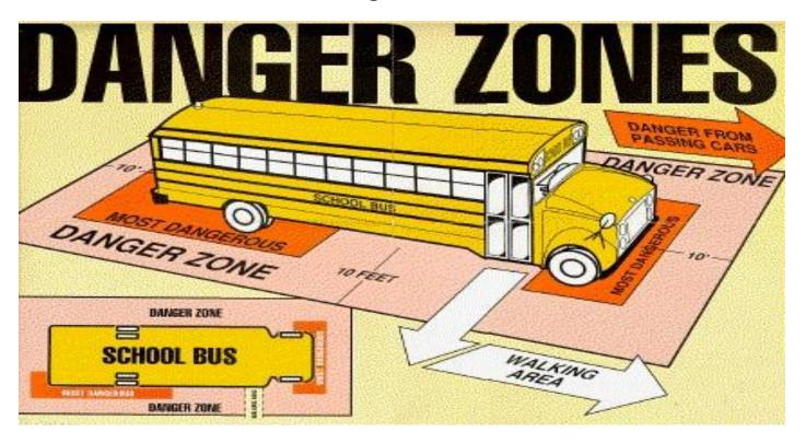
No child should ever be in the pink danger zone. Children leaving the bus should walk straight ahead, away from the bus, for at least 10 feet before turning in either direction. When it is necessary for children to cross in front of the bus, they should walk ten feet from the bus door, (in the direction of the white arrow) before turning toward the front of the bus.
