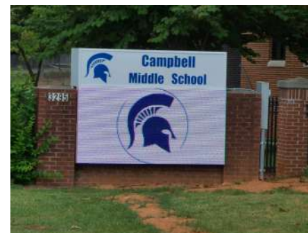
Location: Marietta, GA Year Installed: 2020 Message Sign Pitch: 8mm Display Size: 4ft x 8ft.
