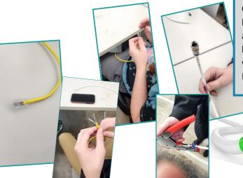
Computer Tech Support students were busy this week learning to make Coaxial and Network cables (Cat5). Students learned proper crimping to make a watertight fit and how to connect RJ45 and RJ45EZ terminals.
