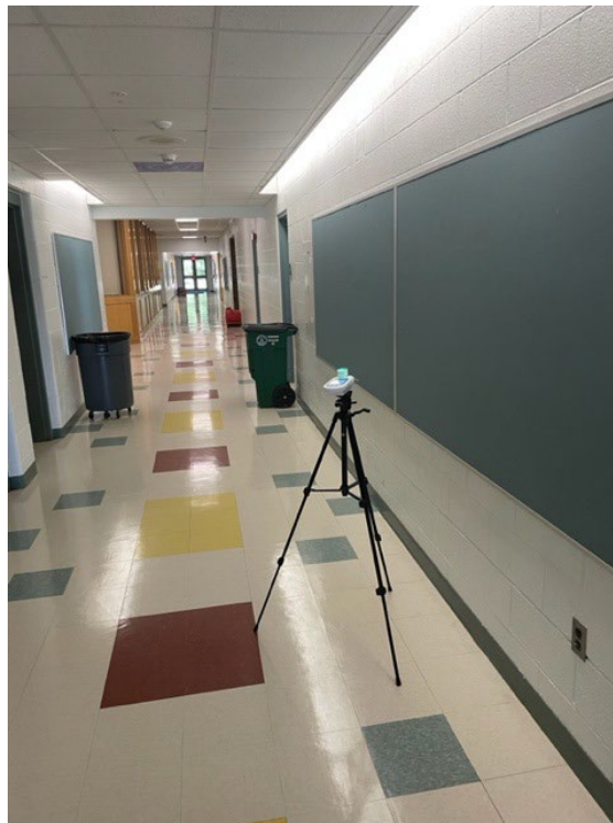
Photograph 2 - Spore trap sample collected at Art Room Hallway. Note: lower wall/cove base previously cleaned.
