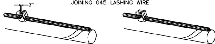
REMOVE ANY SLACK IN THE LASHING WIRE BY MAINTAINING A PULL ON THE WIRE AND TAPPING THE STRAND SHARPLY. THEN FORM THE WIRE OVER THE STUD AND TIGHTEN THE NUT. CUT THE FREE END OF THE LASHING WIRE OFF 3/4\"
