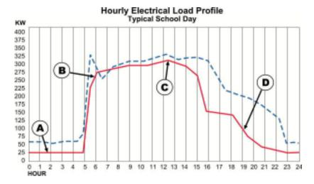
Blue Line (dash) - This indicates a typical electrical use pattern (load profile) that could be found while monitoring any given school day.
