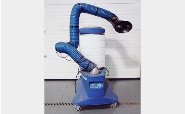
A fume extractor, such as this, can be used to protect from welding fumes.
