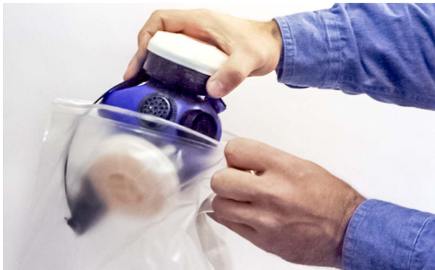
The best storage for an air-purifying respirator is an airtight plastic bag.
