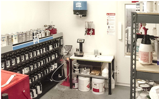
The paint mixing room must be properly ventilated, and well lit for safe operation.
