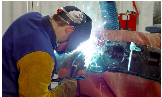
Welding smoke is actually tiny solid particles or particulates. Layers of filter material protect against particulates.
