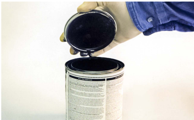
Liquid exposed to the air starts to evaporate, causing vapors. Activated carbon is the usual filter material for protection.
