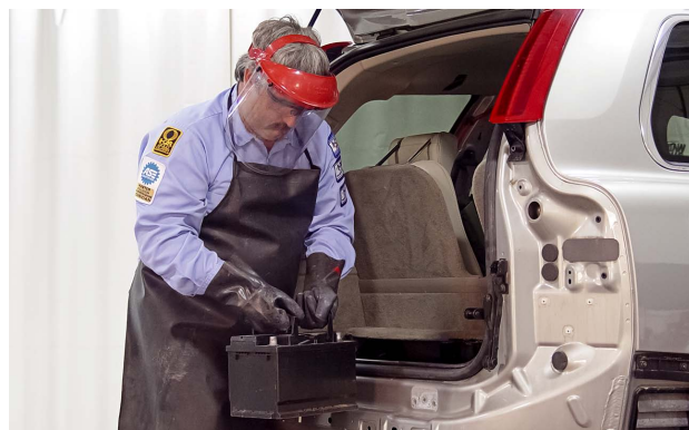
Wearing proper personal protective equipment such as neoprene gloves, goggles, a face shield, and a rubber apron will provide protection from corrosives.
