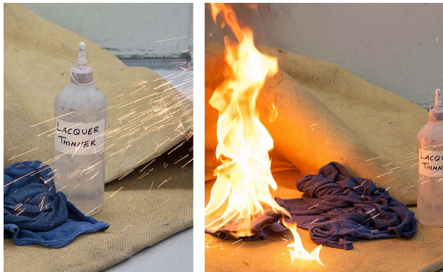
Flammables have a low flash point and must be kept away from sparks to prevent a fire.
