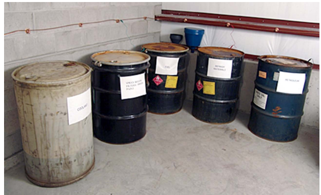
All storage containers should be properly marked and grounded.
