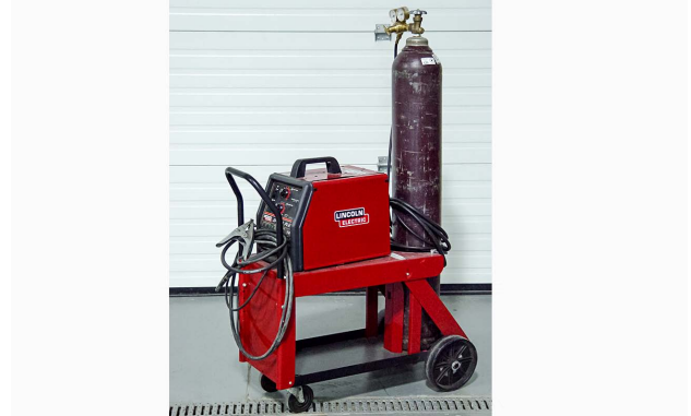
Storing the welding cables properly, such as keeping them off the floor, helps keep the cables in good condition.
