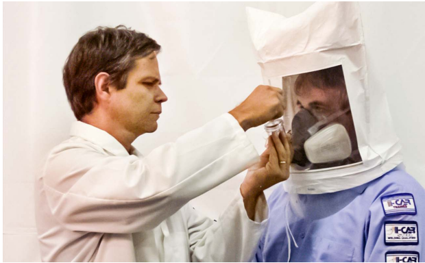
A fit-test involves tasting a particulate mist through the respirator.
