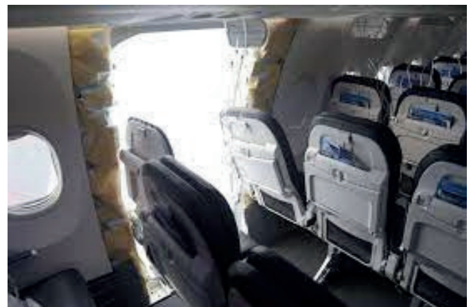
Left: the panel that flew off an Alaska Airlines plane.
