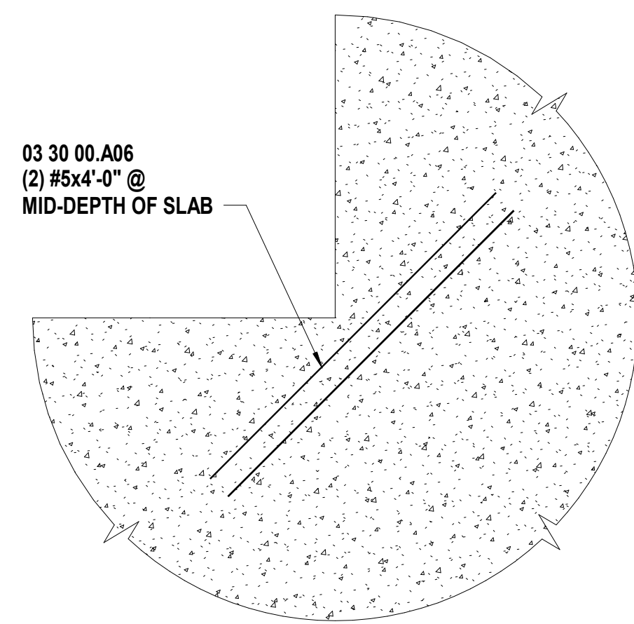
A13 Scale Typical Reinforcing at Re-entrant Corner NTS
