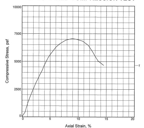
Sample No. 1 Unconfined strength, psf 7055 Undrained shear strength, psf 3528 Failure strain, % 9.0 Strain rate, in./min. 0.050 Water content, % 16.5 Wet density, pcf 133.2 Dry density, pcf 114.3 Saturation, % 92.5 Void ratio 0.4856 Specimen diameter, in. 2.80 Specimen height, in. 5.60 Height/diameter ratio 2.00
