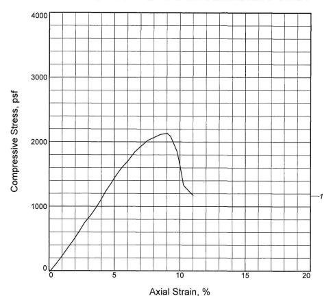
Sample No. 1 Unconfined strength, psf 2134 Undrained shear strength, psf 1067 Failure strain, % 9.0 Strain rate, in./min. 0.050 Water content, % 26.0 Wet density, pcf 114.9 Dry density, pcf 91.1 Saturation, % 82.0 Void ratio 0.8632 Specimen diameter, in. 2.80 Specimen height, in. 5.60 Height/diameter ratio 2.00
