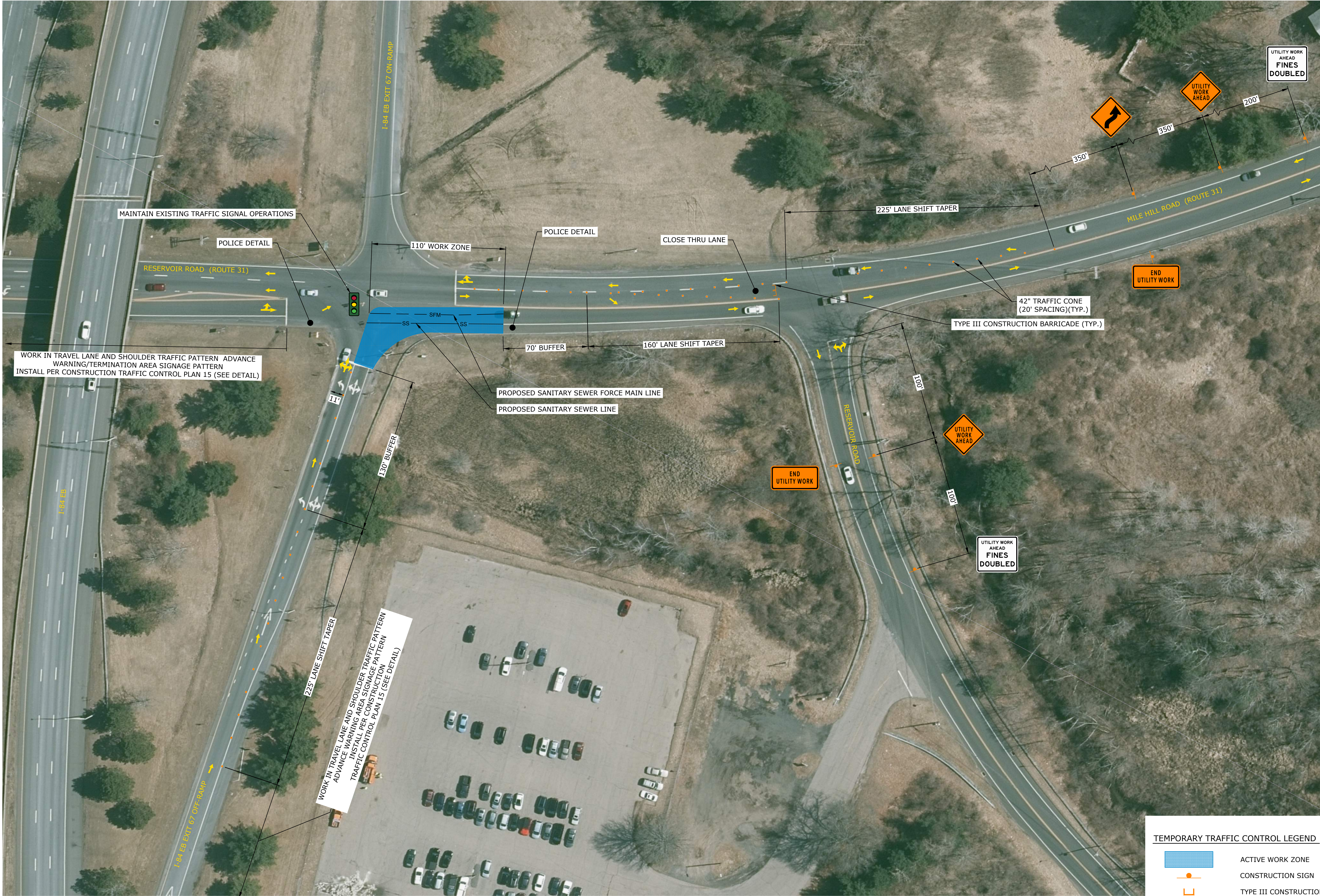
EXIT 67 SEWER EXTENSION TEMPORARY TRAFFIC CONTROL PLAN - PHASE 8 (MON-FRI, 9AM - 4PM)
