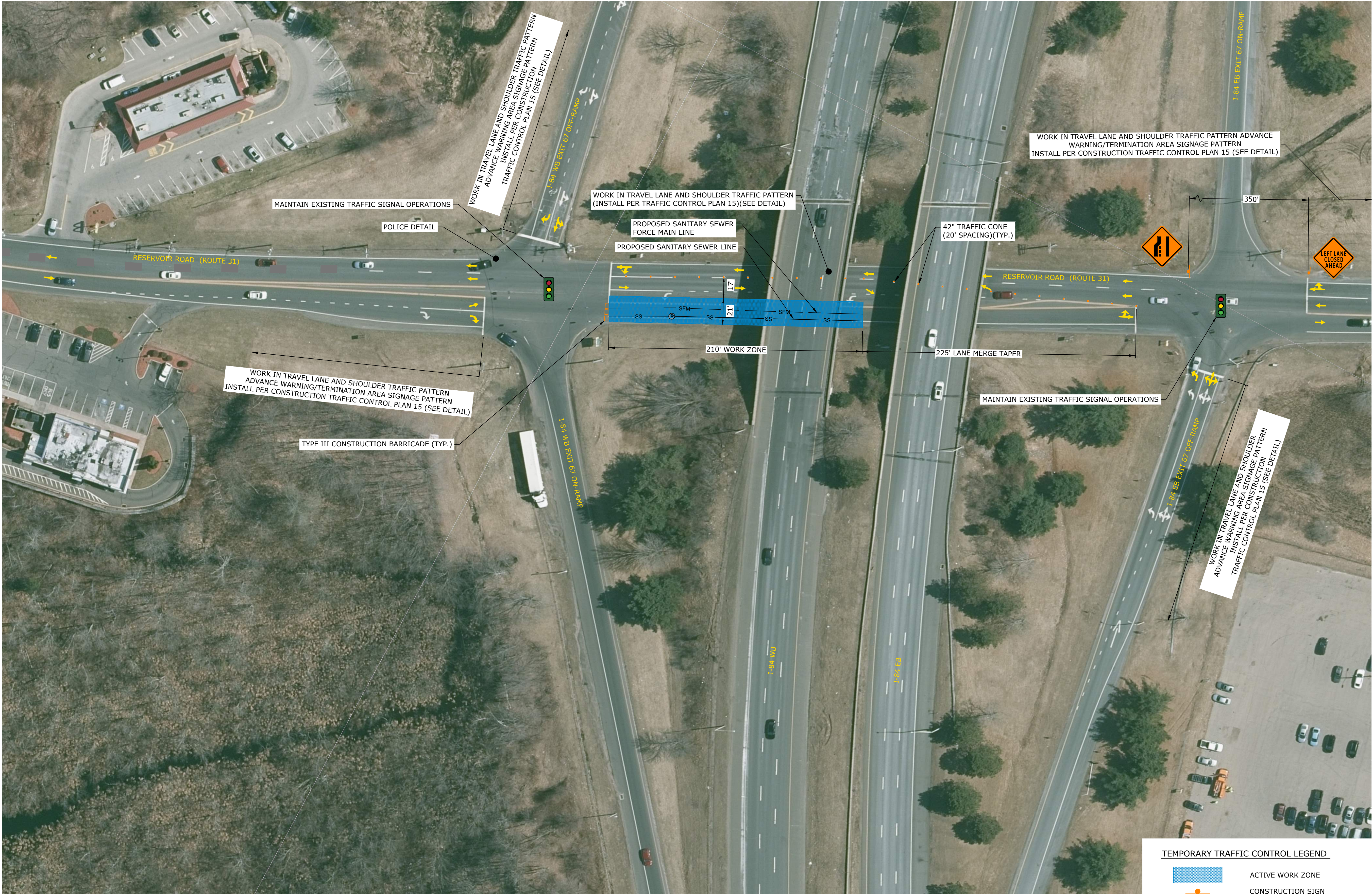
EXIT 67 SEWER EXTENSION TEMPORARY TRAFFIC CONTROL PLAN - PHASE 11 (MON-FRI, 9AM - 4PM)
