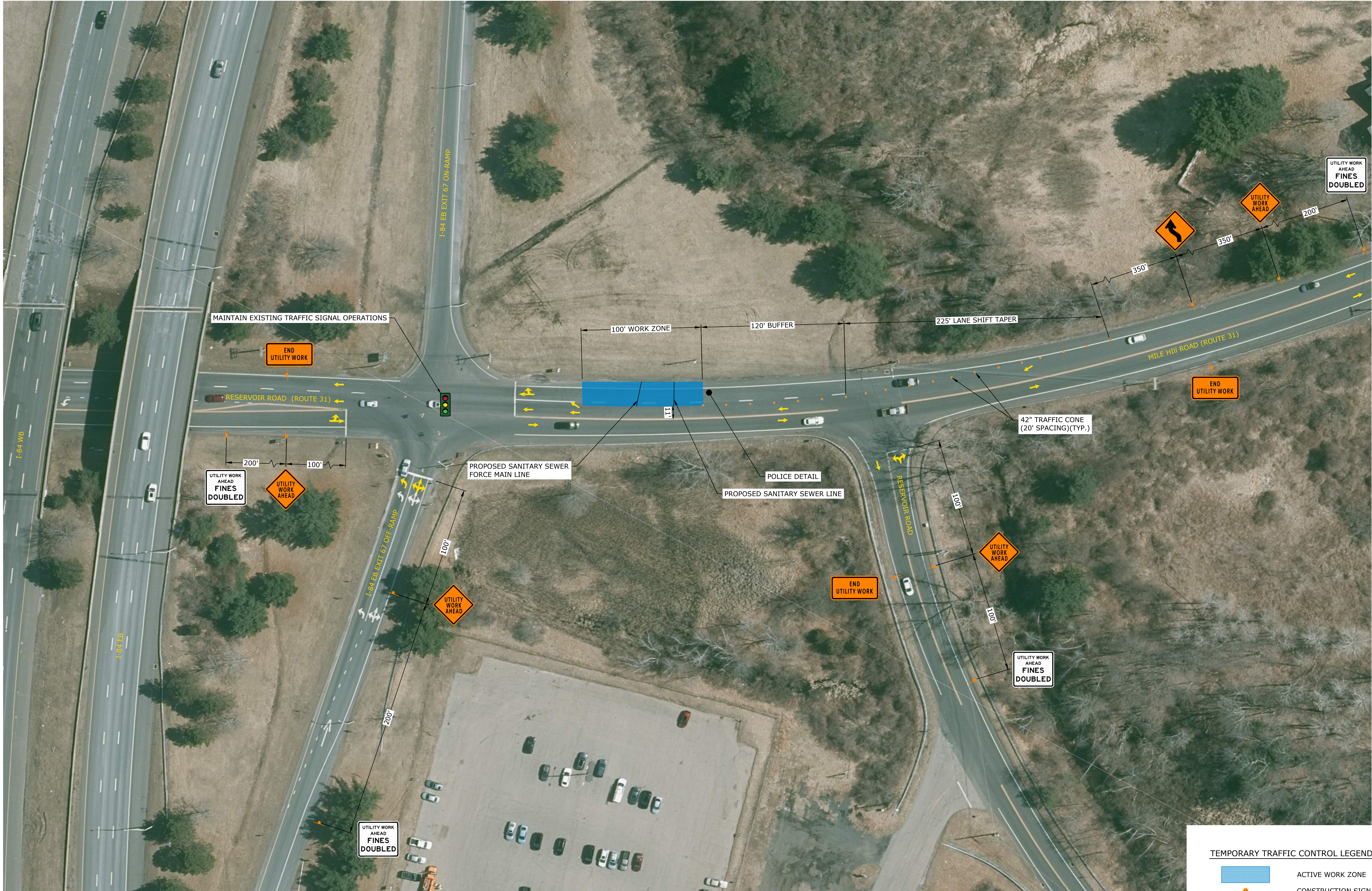
EXIT 67 SEWER EXTENSION TEMPORARY TRAFFIC CONTROL PLAN - PHASE 7 (MON-FRI, 9AM - 4PM)
