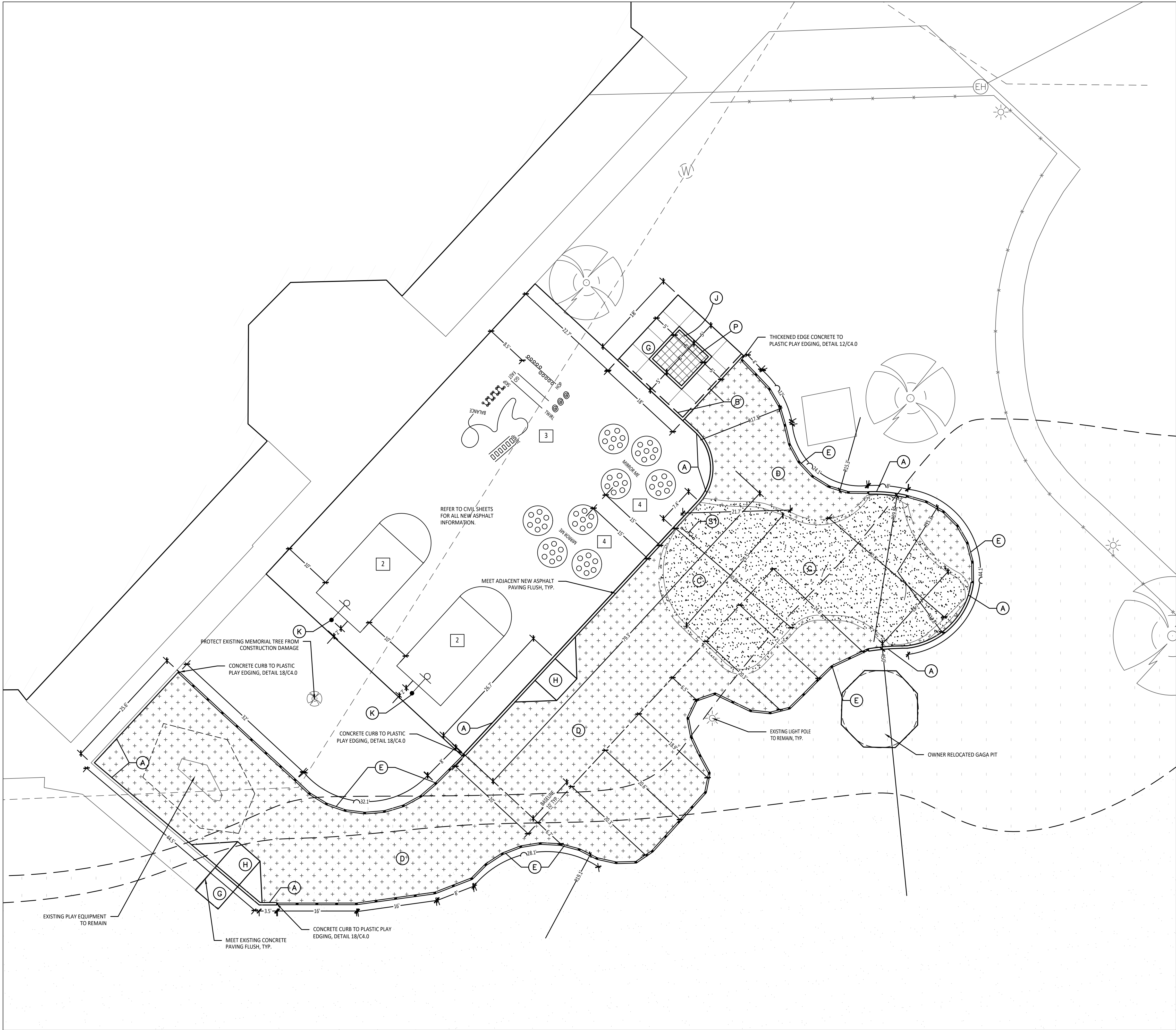
1 Playground Layout Enlargement Plan - Lower Elementary Scale: 1"=10'-0"
