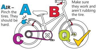
**CHAIN/CRANK** –If there are problems with your gears or if the chain is loose, fix your bike or
