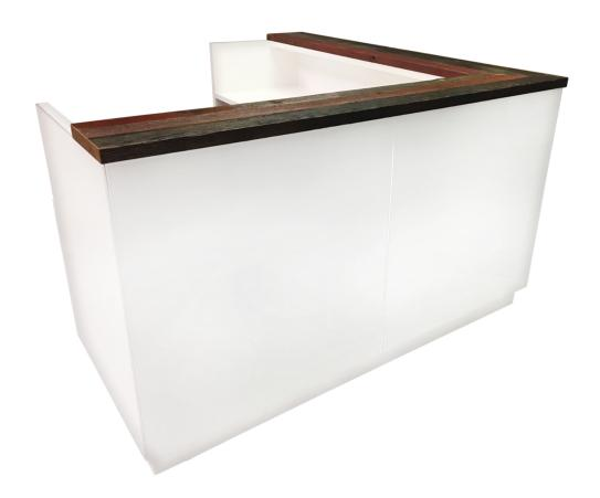
Clad with 1/4" low iron tempered back-painted glass, the Soho reception desk features a reclaimed wood transaction counter and matching file storage fronts. The worksurface is a colorcore matte laminate. Other wood and finish options available upon request.
