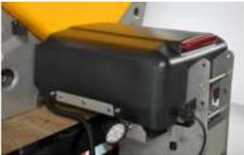
The spinner cable on the 3.5 and 5.0 cu yd POLY HELIXX and the 3.0 through 6.0 cu yd SS HELIXX models produced after 01/20/20 have been updated to a longer cable, making it easier to plug-in when the accessory chute extensions are used. If you have a model prior to this date with difficulties connecting the cable, please contact SnowEx technical service.
