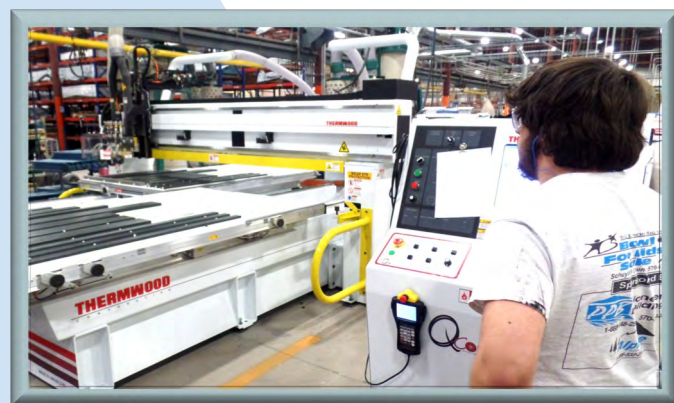
Jacob Strouse monitors a CNC program cutting PVC components for outside furniture products at Highwood USA, Hometown.
