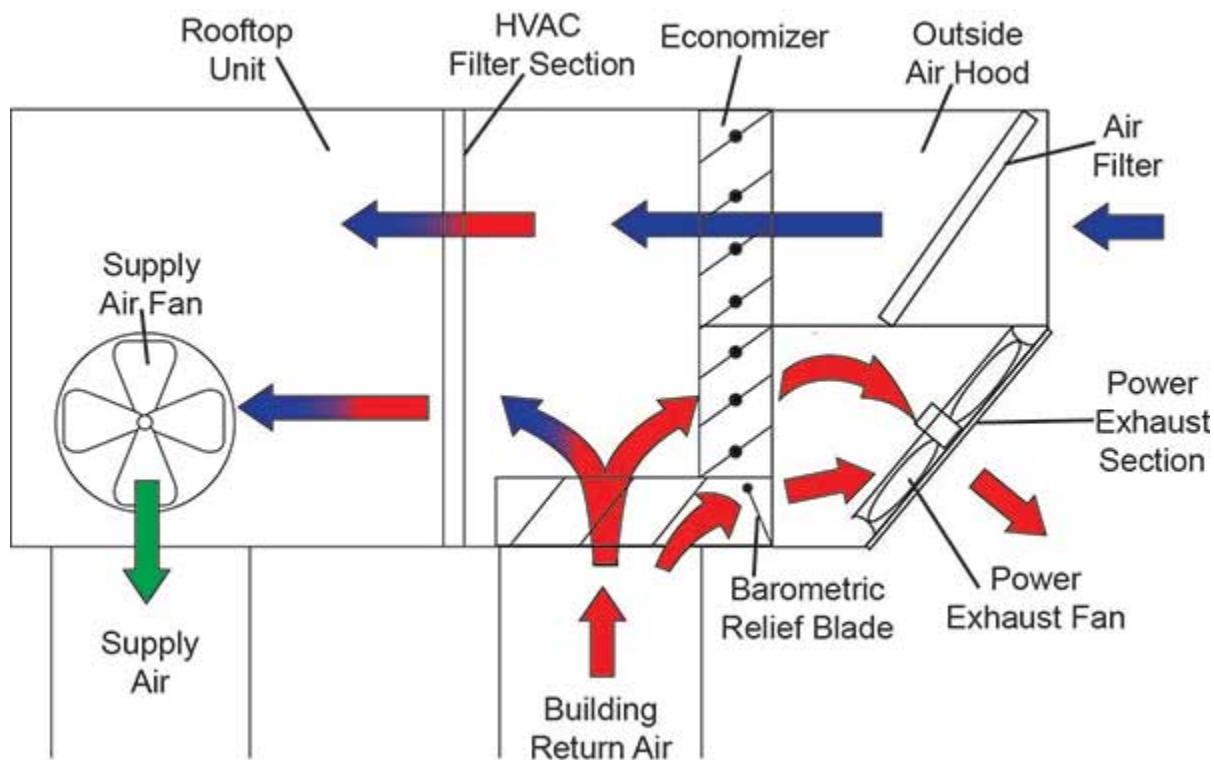
Figure 2 - Typical air handling unit
