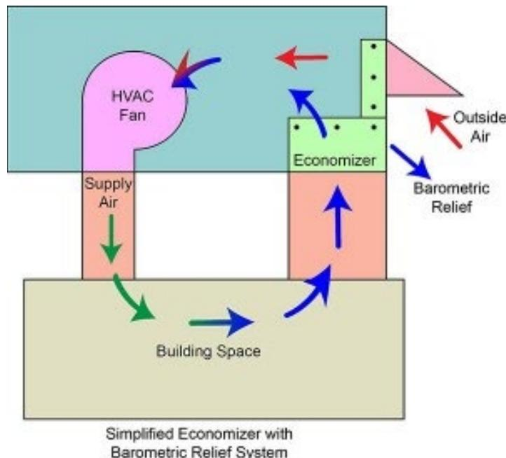
Figure 3 - Proper HVAC pressure relief
