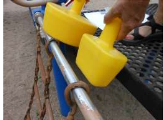
Area of entrapment. Chain climber above deck.
