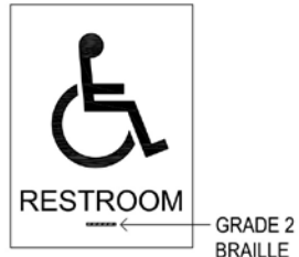
SIGN TYPE F PROVIDE (2) AT ALL INCLUSIVE TOILET AREAS: 6"x8" TO 6"x9" SIGN. THIS SIGN IDENTIFIES THE RESTROOM AREA OFF OF A CORRIDOR FROM EACH DIRECTION (THUS TWO SIGNS).
