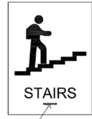
SIGN TYPE H PROVIDE AT ALL STAIRS: 6"x8" TO 6"x9" SIGN
