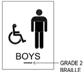
SIGN TYPE E PROVIDE AT ALL GENDER-DESIGNATED TOILET ROOMS: 6"x8" TO 6"x9" SIGN. VERIFY ROOM NAMES, GENDER SYMBOLS, AND WHICH ROOMS SHOULD RECEIVE AN ACCESSIBILITY SYMBOL.
