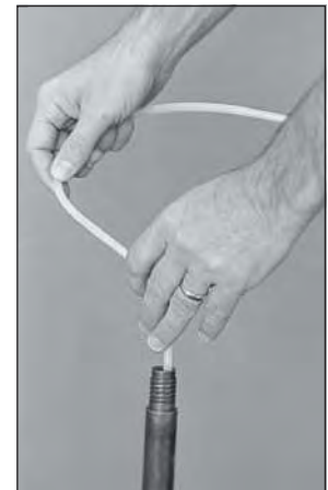
Figure 3. Engaging threads by rotating tubing.
