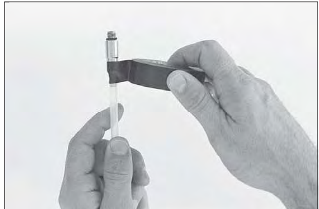
Figure 1. Securing adapter to tubing with tape. NOTE: Tape does not contact soil gas sample.
