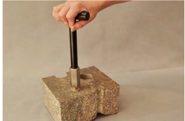
Figure 7. Removing the Vapor Pin™.
