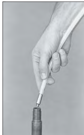
Figure 2. Insertion of tubing and PRT adapter.
