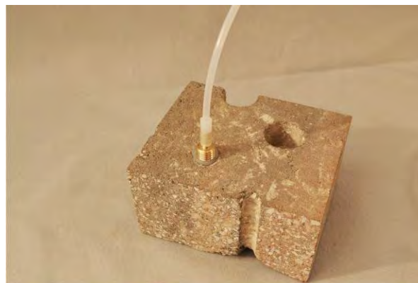
Figure 5. Vapor Pin™ sample connection.
