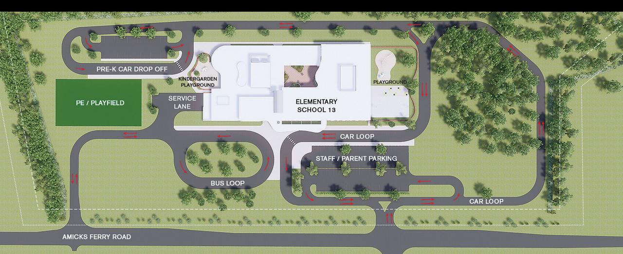
MAIN CAR LOOP STACKING = 1840 LF (SINGLE LANE) PRE-K/K LOOP STACKING = 1450 LF (SINGLE LANE)
