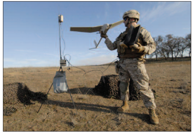
RQ-11 sUAV Raven and antenna
