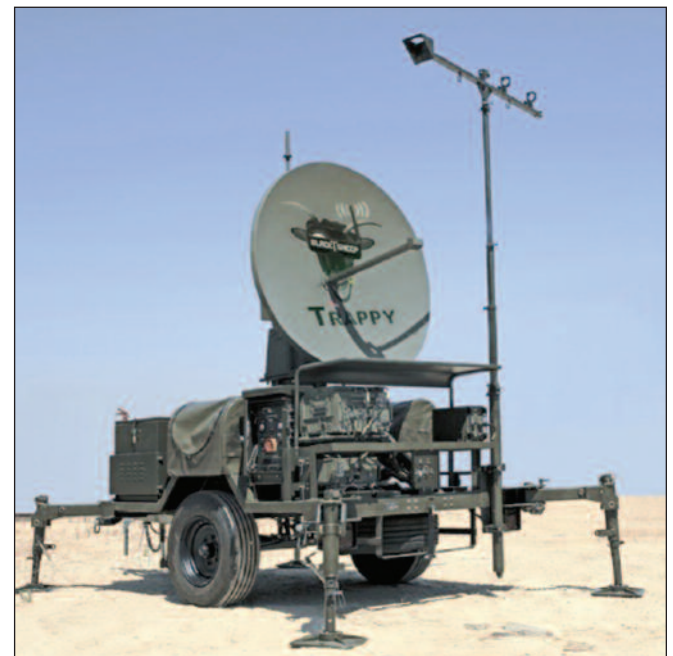
Mobile High power antenna for UAV
