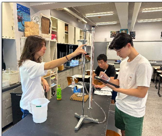
The students hard at work measuring the speed of sound using a resonance tube.
