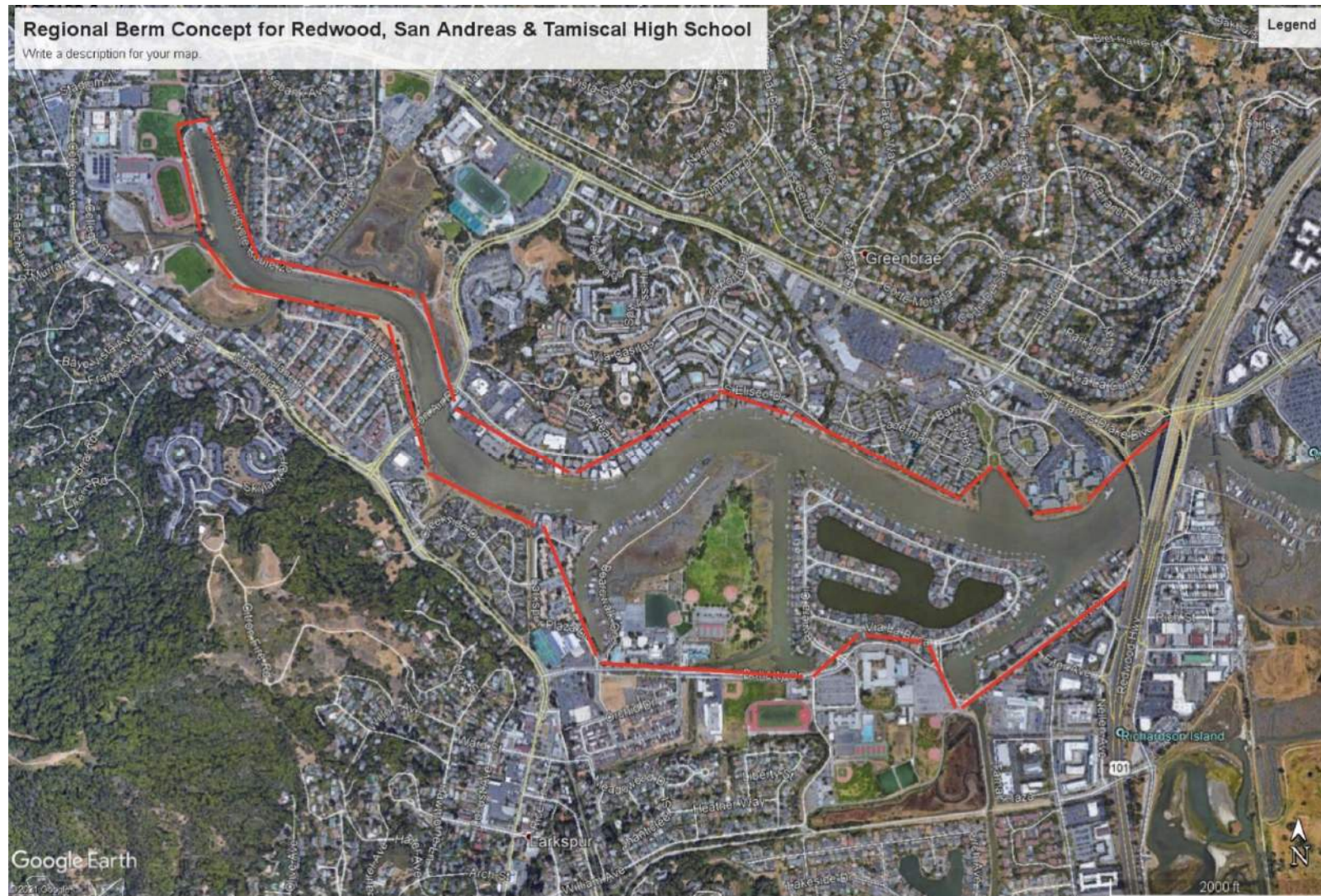
Figure 19: Schematic of regional berm concept to protect Redwood, San Andreas, and Tamiscal High Schools from inundation by the 1% flood event at present and 2120 sea levels. This concept is based on the Cardiff Living Shoreline hybrid solution concept for sea level rise adaptation and is a far-term solution with many regional stakeholders required.
