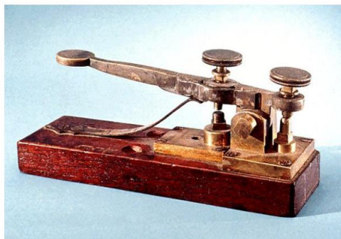
The telegraph key, pictured above, was pressed repeatedly to send a pattern of long and short signals. This key was used by Samuel Morse to send the famous message "What hath God wrought?" in 1844.
