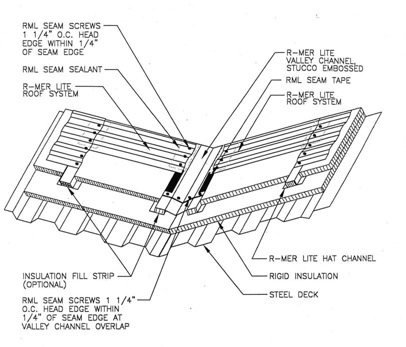
\*NOTE: ALL FASTENERS IN VALLEY COATED WITH SEALANT
