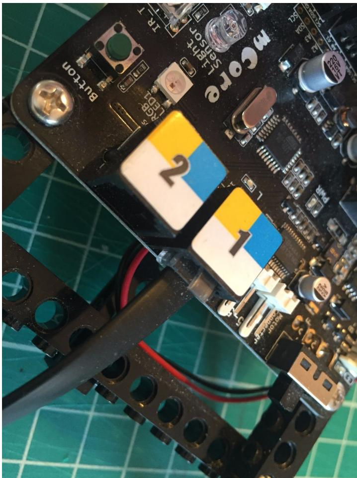
Attach the cable to Port 1 on the mCore.
