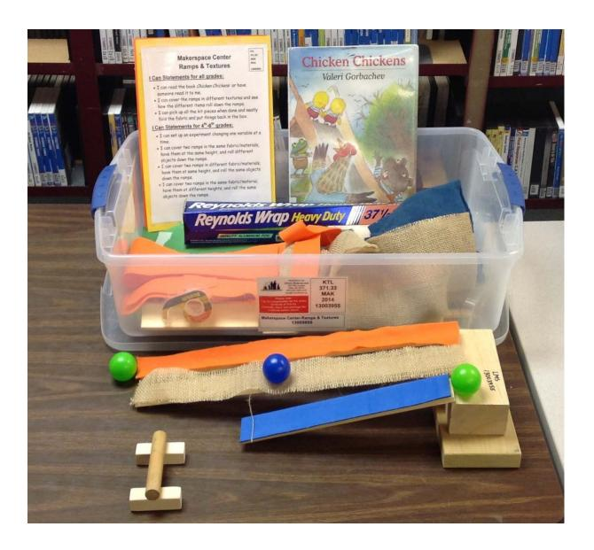
This kit includes items needed to set up a makerspace center for young students to experiment with rolling different items down ramps covered with different materials: includes wooden blocks, ramps and balls, plastic balls, marbles, cylinders, toy cars, burlap, felt, and more.
