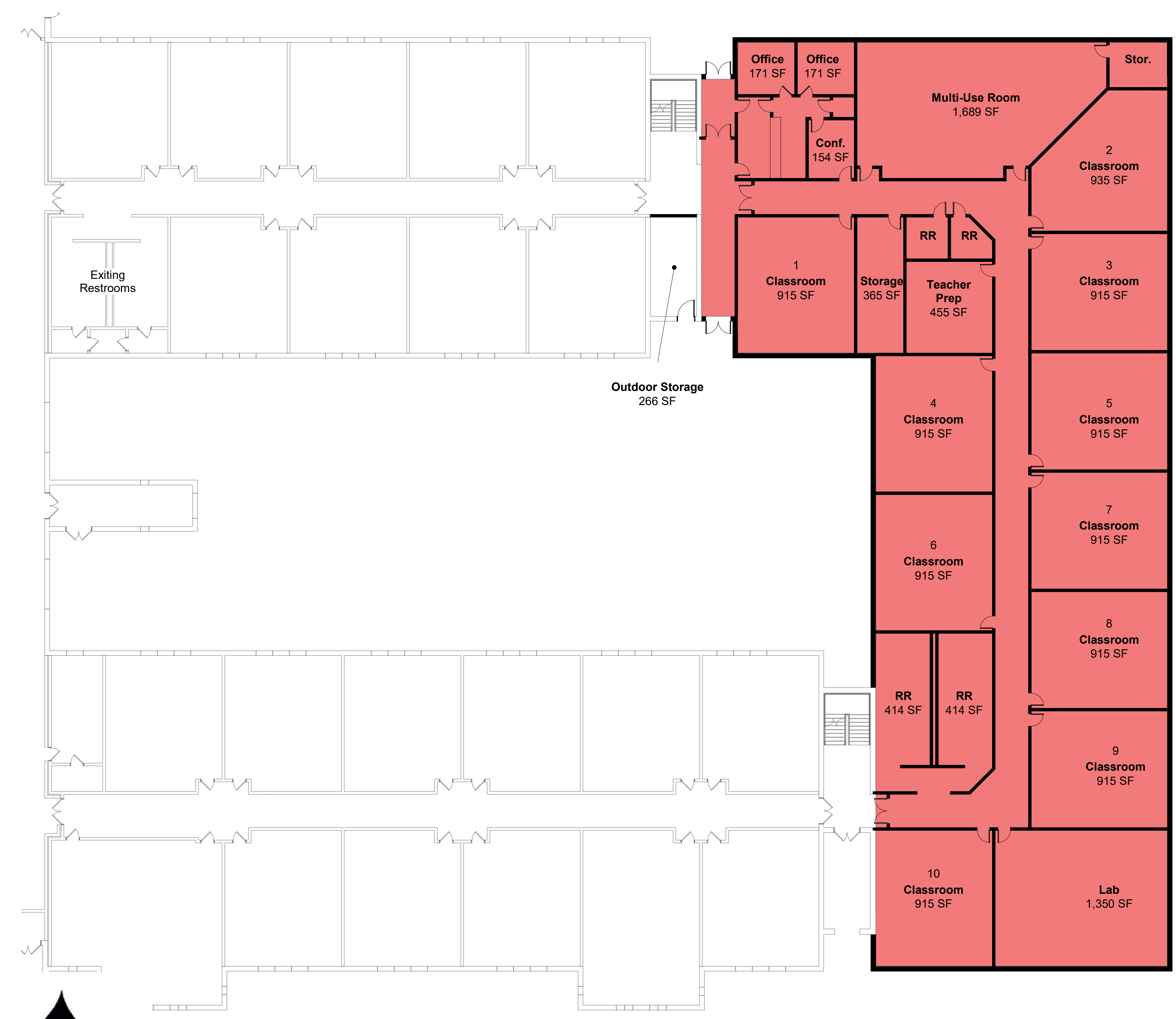
NORTH 3-12 Classroom Addition First Floor Plan 1/16" = 1'-0" 0 8 16 32
