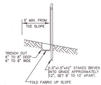
SEDIMENT CONTROL FABRIC TO BE A GEOTEXTILE MATERIAL TREATED TO RESIST DEGRADATION FROM EXPOSURE TO SUNLIGHT.
