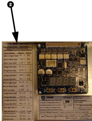
1. To check status, configuration, or to change settings on the engine board with the power on the unit, detach the low voltage access lid and look or reach through the low voltage access panel.
