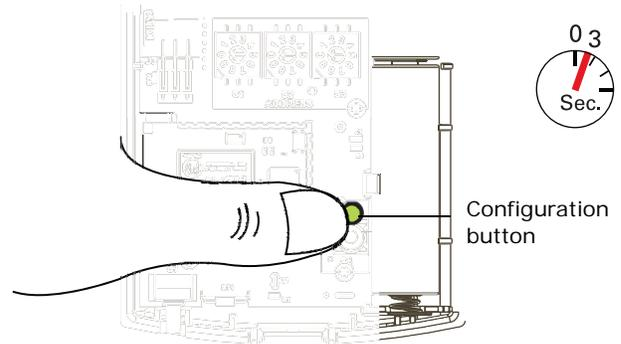
The display will change to configuration mode. When the sensor is in configuration mode, a wrench symbol appears on the display and the menus are separated by lines, as illustrated below.
