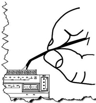
To connect wires to the UC400 controller or the expansion modules:
