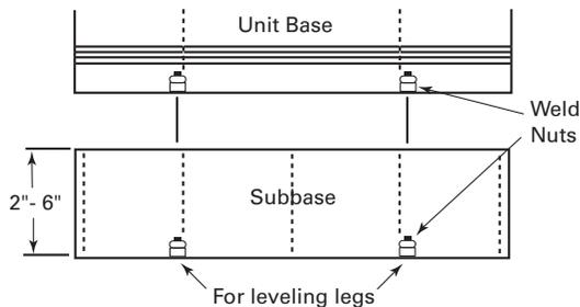
2. Set the unit on the subbase and fasten with four, 3/8 in. x 16 ft x 1 in. hex head cap screws and 3/8 in. lock washers.
