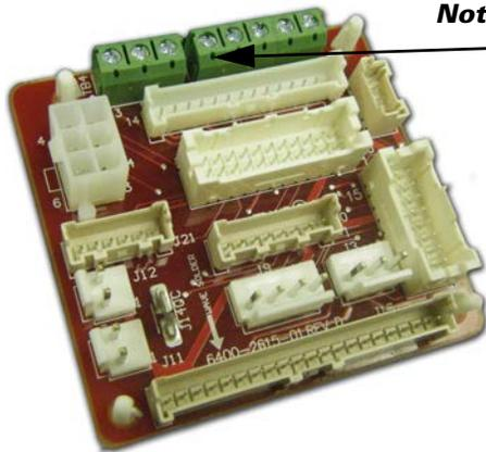
**Note:** Customer Low-Voltage Interface for Fan Speeds, Variable Fan Speed, and 24 Vac Supply
