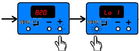
**Example 3.** We wish to double check to see if the value of “820 rpm” has been saved.
