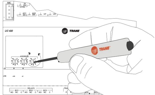
Use a 1/8 inch (3.2 mm) flathead screwdriver to set rotary address dials. Dials rotate in either direction.
