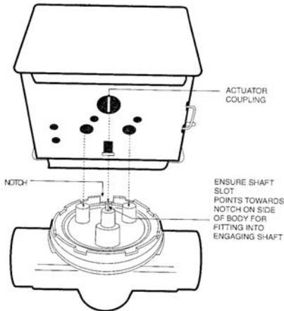
4. Install body valve into pipe.
