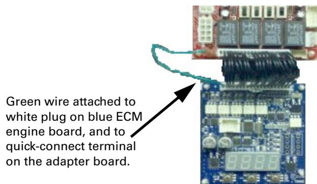
4. Ensure that the new ECM engine controller is configured to match the ECM engine configuration label that is present on the unit. It is necessary to configure the ECM engine board to avoid improper
