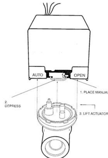
**Figure 22. Installing isolation valve**
