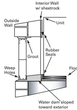
Figure 10. Flanged wall box installation in 2-in. curtain wall
