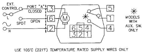
**Figure 19. Wiring for modulating valve actuator**
