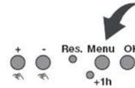
1. Press the **Menu** button until the display screen is blank (time not showing) and **24h** or **am/pm** is blinking in the upper left corner of the screen.
