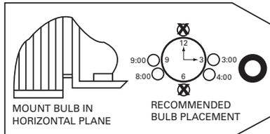
**Note:** Depending on the controls package ordered with the unit, not all installations will require mounting the frost stat bulb.
