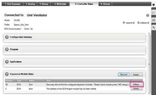
Notice one ECM type is configured at address 99, but no ECM is found at that address. Also, notice that another ECM has been found with an address of 0. When this situation occurs, Tracer TU displays a Softset... button you can use to configure the engine module address.
