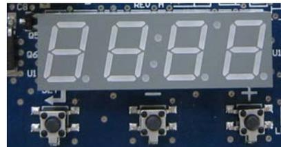
The ECM engine board contains a four-digit, seven-segment display that is used to present information in a format close to real-world language, while having a small-form factor. Most characters are immediately recognizable; however, please consult [Table 9](#) and [Table 10](#) for the graphical representation of each alphanumeric character.
