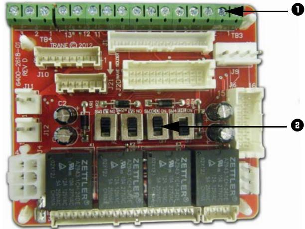
1. Customer Low-Voltage Interface for Valves, Electric Heat, Dampers, Fan Speeds, Variable Fan Speed, and 24 Vac Supply
