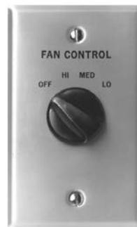
The fan speed switch can be used to provide simultaneous fan speed customer requests in addition to external controller fan speed request. The wall-mounted option is low-voltage and has three 24-volt relays using a factory-wired transformer and relays to control the fan motor.
