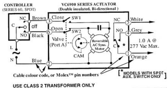
The typical floating controller is an SPDT controller with a center-off position. On a change in temperature from the set point, the controller will close the normally open (NO) or normally closed (NC) contacts, driving the valve to an intermediate position until a further change at the controller.
