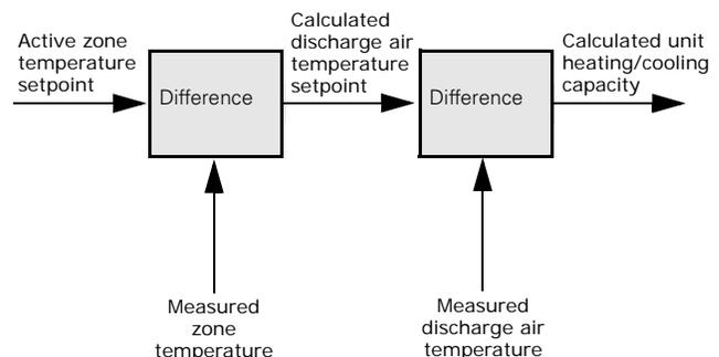
If the discharge air temperature falls below the discharge air temperature low limit setpoint, (configurable using the Tracer TU service tool), and the cooling capacity is at a minimum, the available heating capacity is used to raise the discharge air temperature to the low limit (refer to the following section, “Discharge Air Tempering (UC400):”).
