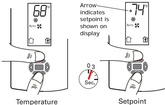
**Locking or Unlocking Settings.** You can lock or unlock the setpoint, system, or fan setting to prevent changes.
