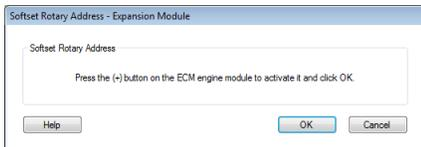
2. Prior to clicking OK, activate the engine module using the **(+)** button on the ECM engine board in the control box.
