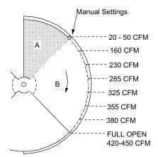
Inside the lower section, locate the circular calibration plates as noted in the drawing ("A" is fixed, "B" is movable). Remove the screw shown by the arrow from "Manual Settings."
