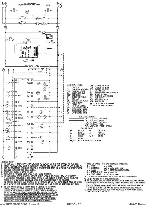
Figure 7. Typical Wiring Schematic for Heat Pump Single Phase Power
