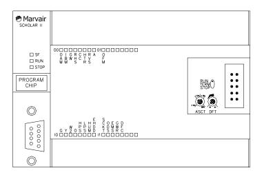
or thermostat. The first four outputs, from left to right, are connected to a 230 VAC supply and thus provide 230 VAC when energized. These outputs are:
