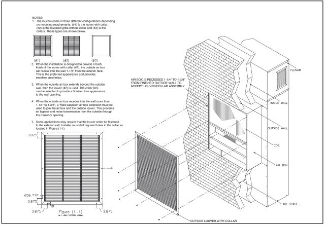
Figure 2. Installation of Louver/Collar Assembly to Air Box
