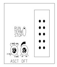
The micro switch has three positions – **RUN**, **TERM & STOP**. The switch should be in the **RUN** position during normal operation. **Term** is for operation from a remote terminal. **Stop** is no output/non-operational.
