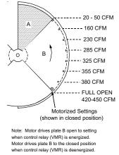
Operation is the same for the "Motorized" and "PowerVent" systems. Inside the lower section, locate the circular calibration plates as noted above in the drawing ("A" is fixed, "B" is movable). Remove the screw shown by the arrow from "motorized settings."
