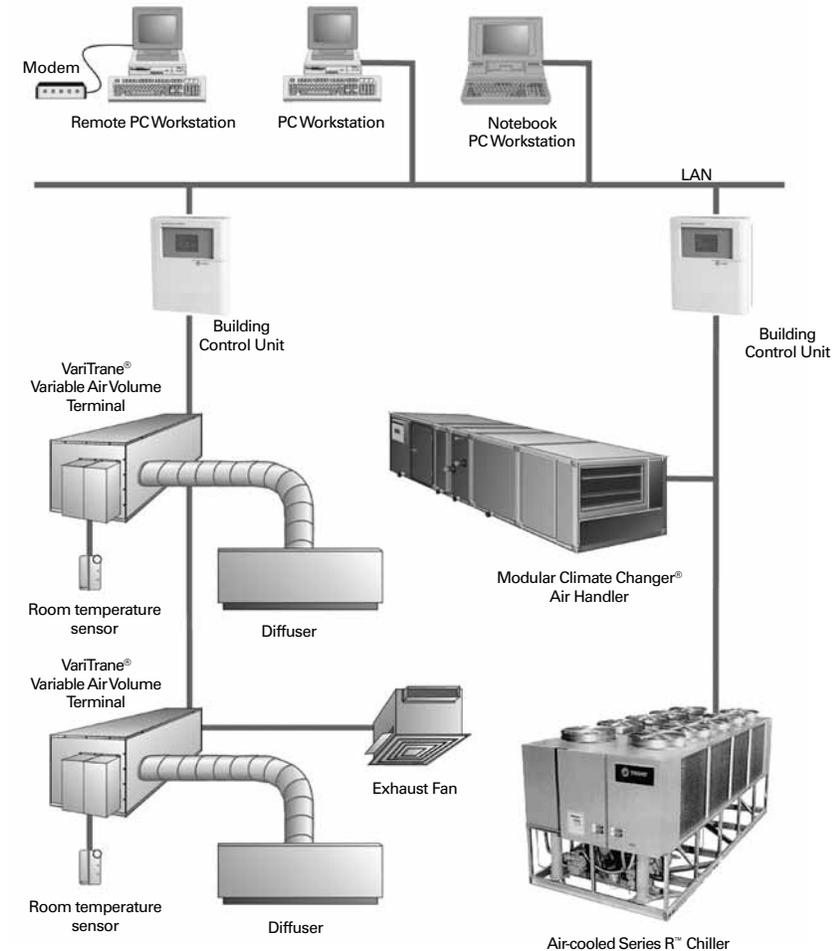
and leaving evaporator water temperatures and outdoor air temperature. Over 60 individual diagnostic codes can be read by the Tracer system. In addition, the Tracer system can provide sequencing control for up to 25 units on the same chilled water loop. Pump sequencing control can be provided from the Tracer system. Tracer ICS is not available in conjunction with the remote display or the external setpoint capability.
